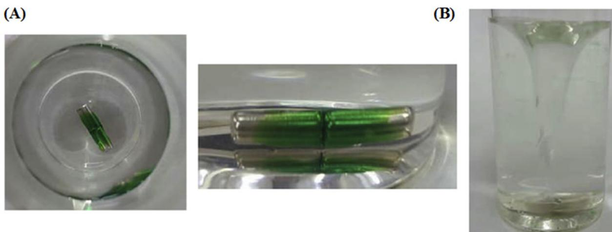
**Fig. 5.** Images of a stir-bar coated with the trihexyltetradecylphosphonium tetrachloronickelate(II) ( $[P_{6,6,6,14}]^+ [Ni(hfacac)_3]^-$ ) MIL (A), and the dispersion of the MIL during a SBDLME procedure (B). Reprinted with permission from reference [45].
