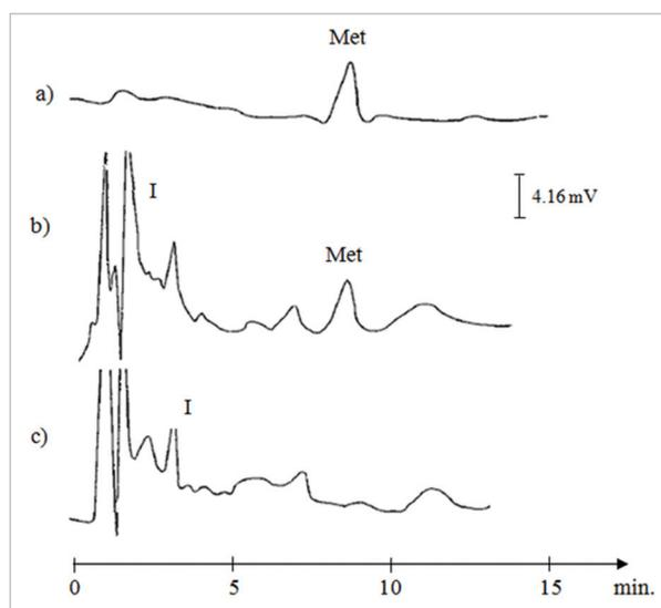
**Figure 3.** Chromatograms obtained from a SPE of 100 ml water at concentration of 1  $\mu\text{g L}^{-1}$  Methidathion, a) HPLC grade water, b) drinking water spiking c) drinking water without spiking. Met= methidathion, I= interfering compounds. "Nucleosil". Precolumn extraction.
