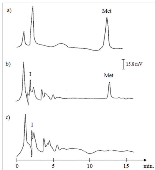
**Figure 2.** Chromatograms obtained from a SPE of 250 ml water at concentration of  $0.6 \text{ mg L}^{-1}$  Methidathion, a) drinking water b) HPLC grade water c) drinking water without spiking. Met= methidathion, I= interfering compounds.
