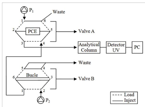
**Figure 1.** Experimental setup for the pre-concentration, extraction and on-line analysis (PCE = precolumn, UV = ultraviolet, PC = personal computer).
